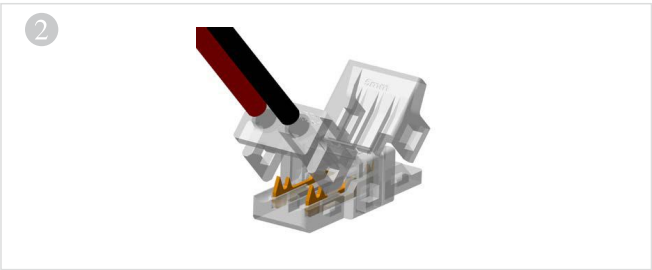
2. Cut the wire according to the required length, and insert it into the wire slot of the connector to the bottom. Close the flip cover and lock both sides of the buckle, using tools like electrician pliers if possible.
